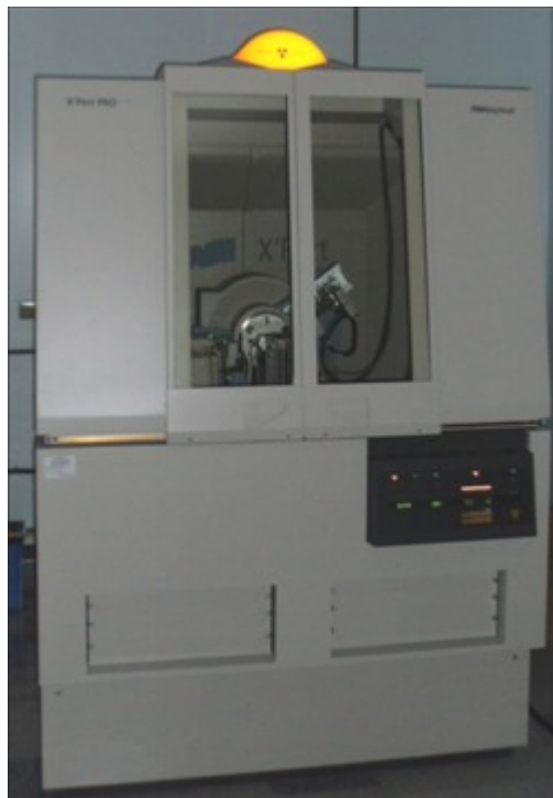
Figure 3.5 Photographic view of X-ray powder diffractometer used in this study
