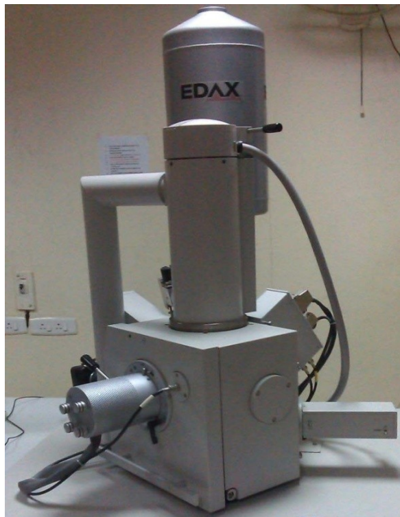
Figure 3.6 Photographic view of scanning electron microscope used in this study
