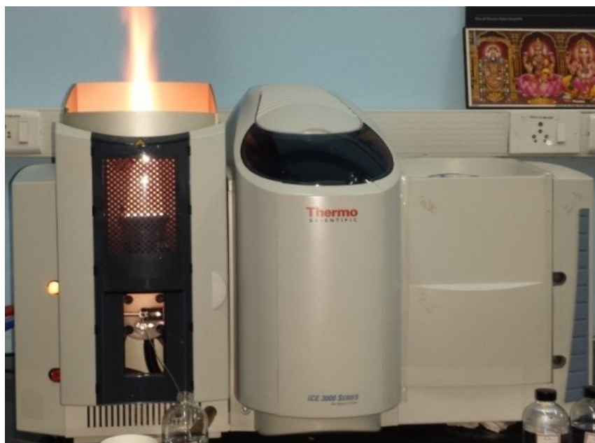
Figure 3.1 Photographic view of atomic absorption spectrometer used in this study
