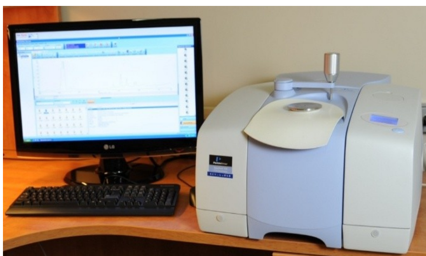
Figure 3.4 Photographic view of Fourier transform-infrared spectrometer used in this study
