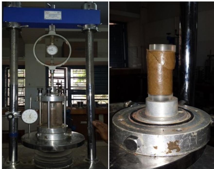
Figure 3.8 Photographic view of unconfined compressive strength test conducted in this study
