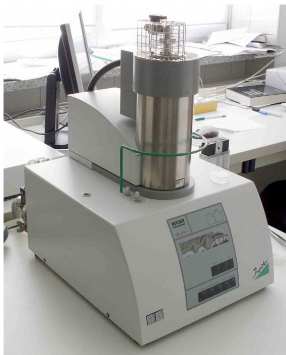
Figure 3.3 Photographic view of thermo gravimetric analyzer used in this study
